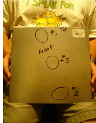
Figure 26, Post Combat Arrow Test Front Side
