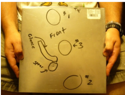
Figure 31, Post Spear Impact Front Side
