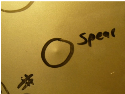
Figure 35, Post Spear Impact Back Side
